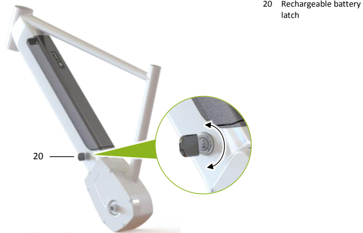
Figure 8 Rechargeable battery latch
