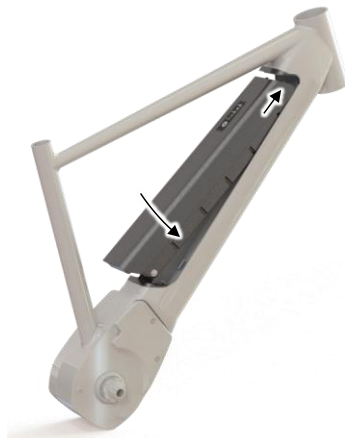
Figure 7 Insertion of the rechargeable battery
